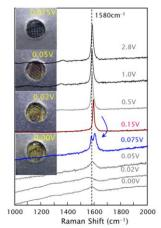
Operando studies of an anode. The graphite G-band Raman peak also changes, indicating intercalation and then a peak-splitting reflecting the intercalation penetrating to interior layers, rather than just the boundary layers.
