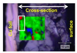
Raman mapping and imaging enables the study of the distribution of materials on electrode surfaces, or across cross-sections. The resulting data can be quantified, giving metrics such as fraction estimates and particle statistics.
